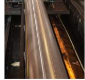
Electric resistance welding (ERW – up to a diameter of 610 mm) and submerged arc welding (SAW – up to a diameter of 2540 mm) technologies are used to produce pipe from different grades of carbon steels. The in-house application of high performance protective coatings and linings to steel pipe is an essential ingredient when years of trouble-free pipeline service is a pre requisite.
